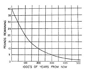
A radioactive substance decays into another element. The curve in the graph above shows how much of the radioactive substance remains over time. From the graph, estimate the half-life of the substance.
